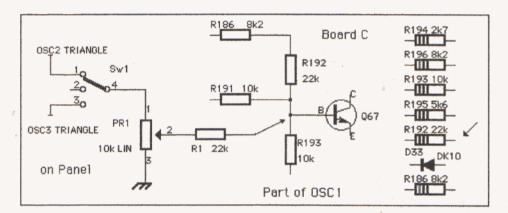
Each sync circuit comprises a single pole centre off switch to select the other two oscillator outputs (taken from the top of a level pot), this is taken to an extra pot and the wiper feeds a resistor connected to the Oscillator hysteretic switch to alter its threshold. This has to be "flown" onto the pcb and soldered to the end of the 22k resistor as indicated. The pcb layout of each Oscillator is identical at the top of the board.
