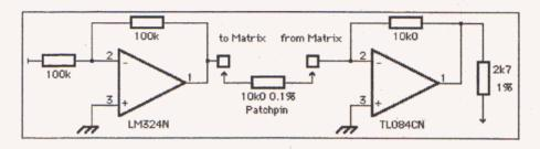
This also achieves True Summing of the patchboard (the standard circuit is a weighted average). The circuitry may be built using quad op amps and mounted close to the matrix patchboard. The IC driving the matrix must be capable of operating into the load of several pins in parallel without becoming unstable. The power supply may be taken from the nearest convenient point, don't forget some decoupling capacitors across each rail.
