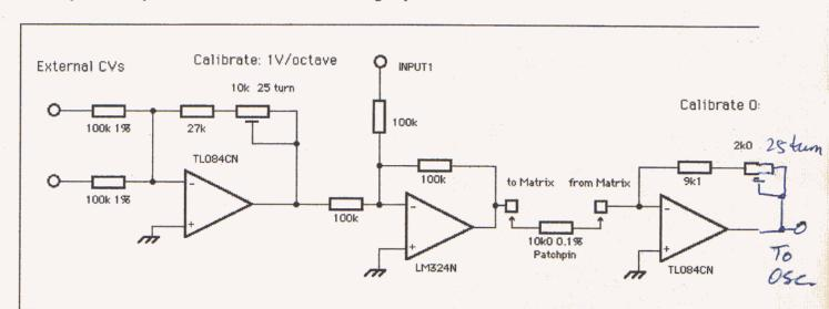
Although the Trigger Key is specified as being a +4V voltage it should really be a **switch to +4V**, here's a simple interface circuit that will accept external +10V Gates or LFO waveforms and still function with
