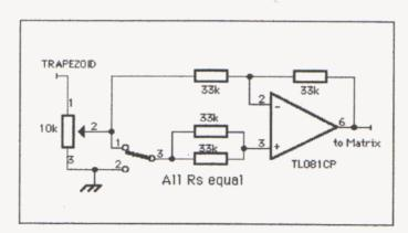
Make all 4 resistors the same value, eg 33k; this just saves having to get two resistors of exactly double values, it will work with whatever you have handy. When the switch is at ground you have a normal inverter configuration: gain = -1; when the switch is connected to the pot wiper the gain = -1 + 2 = +1.
