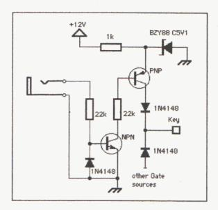
This circuit will trigger the Envelope Shaper from any external voltage sufficient to turn the NPN transistor on (i.e. >1V) and will protect from gates exceeding the power rails. WARNING: Improper Key interfacing may cause cycling or incorrect voltage output levels of the Envelope Shaper and may even damage it.
